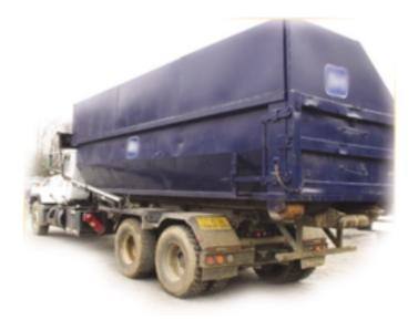
Section 393.134 is not, however, applicable to the operation of hoist-type equipment (or hoist equipment) as described in American National Standards Institute (ANSI) publication ANSI 2245.1. Hoist-type equipment should be considered separate and distinct from roll-on/roll-off equipment and, therefore, not subject to § 393.134. Containers transported on hoist-type equipment must be secured in accordance with the general securement rules.
