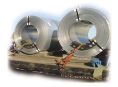
The rules in this section apply to the transportation of one or more metal coils which, individually or grouped together, weigh 2,268 kg (5,000 lbs) or more. Shipments of metal coils that weigh less than 2,268 kg (5,000 lbs) may be secured in accordance with the general cargo securement rules.
