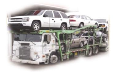
This portion of the new standards applies to the transportation of automobiles, light trucks, and vans which individually weight 4,536 kg (10,000 lbs) or less. Vehicles which individually are heavier than 4,536 kg (10,000 lbs) must be secured in the same manner as heavy vehicles, equipment and machinery (see the rules under /393.126).
