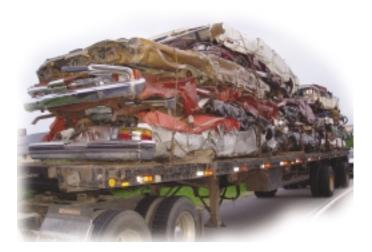
The transportation of vehicles such as automobiles, light trucks and vans that have been flattened or crushed is covered by these requirements. The transportation of automobiles that are flattened or crushed in a crash or accident, as opposed to being intentionally flattened or crushed in preparation for transportation to recycling facilities, is not subject to these requirements. However, vehicles damaged in a crash or accident are subject to the general cargo securement requirements.
