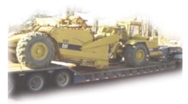
These requirements are applicable to the transportation of heavy vehicles, equipment and machinery which operate on wheels or tracks, such as front end loaders, bulldozers, tractors and power shovels and which individually weigh 4,536 kg (10,000 lbs) or more. Vehicles, equipment and machinery which is lighter than 4,536 kg (10,000 lbs) may be secured in accordance with these rules, the rules for automobiles, light trucks and vans, or the general freight requirements.
